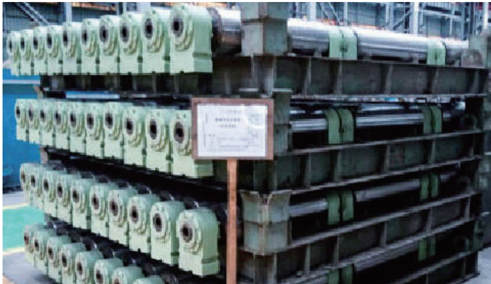
整修連鑄機 SEGMENT 輥輪 Reclaimed rollers for CCM segment
