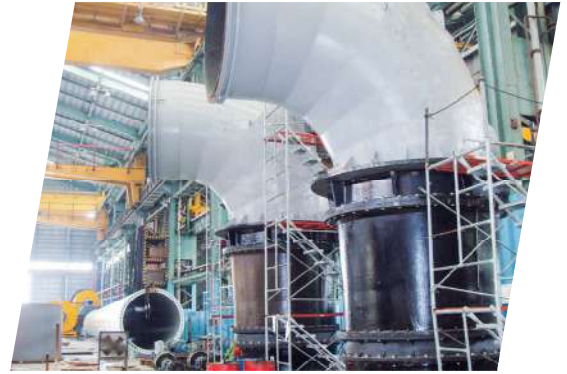
建國抽水擴建站 抽水機於中機廠內組裝 Jianguo pump station Assembling in CSMC
