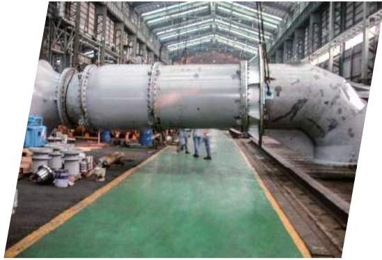
景美抽水站 抽水機於中機廠內組裝 Jingmei pump station Assembling in CSMC
