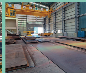
鋼板室內儲區 室內面積：最大 75m(長)x20m(寬) 起重能力：最大 20 噸 Steel plate indoor storage area Capacity of indoor storage area: max. 75m (L) x20m (W) Capacity of lifting for steel plate: max.20 ton
