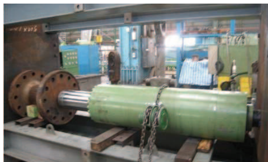
中鋼 W3 油壓缸試壓 Ø280mmx200mmx650 CSC CSC W3 Hydraulic Cylinder Pressure Test Ø280mmx200mmx650
