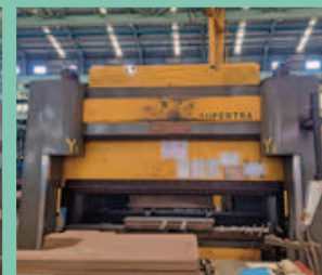
400 噸油壓折床 折床能力：最大 400 噸 400ton Hydraulic bending machine Capacity of bending force for steel plate: max.400 ton
