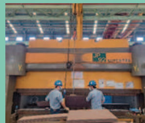
500 噸油壓折床 折床能力：最大 500 噸 500ton Hydraulic bending machine Capacity of bending force for steel plate: max.500 ton
