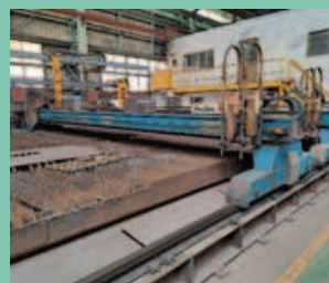
電離子切割機 切割床台尺寸：最大 50m(長)x9m(寬) 起重能力：最大 20 噸 PLASWA cutting machine Capacity of cutting table for steel plate: max. 50m (L) x9m (W) Capacity of lifting for steel plate: max.20 ton
