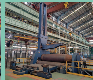
四軸捲板機 捲板能力： 100mm(厚)x4,000mm(寬)x5,250mm(直徑) Bending roller with 4 rollers Capacity of cold bending for steel plate :100mm(T)x4,000mm(W) x5,250mm(Dia.)
