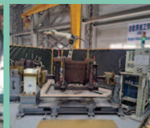
自動焊接工作站 Robotic Welder Station 40mm(T)x3,500mm(W) x6,000mm(Dia.)
