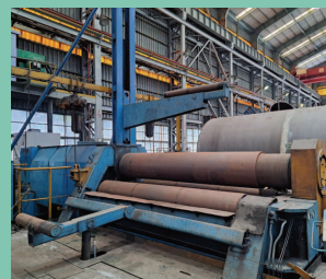
四軸捲板機 捲板能力： 40mm(厚)x3,500mm(寬)x6,000mm(直徑) Bending roller with 4 rollers Capacity of cold bending for steel plate: 40mm(T)x3,500mm(W) x6,000mm(Dia.)
