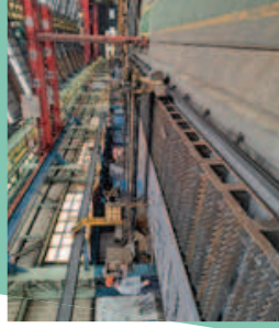
CNC 火焰切割機 切割床台尺寸：最大 45m(長)x3m(寬) 起重能力：最大 20 噸 CNC flame cutting machine Capacity of cutting table for steel plate: max. 45m (L) x3m (W) Capacity of lifting for steel plate: max.20 ton
