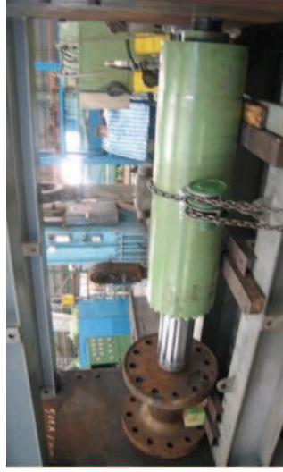
中鋼 W3 油壓缸試壓 Ø280mmx200mmx650 CSC CSC W3 Hydraulic Cylinder Pressure Test Ø280mmx200mmx650
