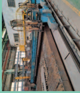
電離子切割機 切割床台尺寸：最大 50m(長)x9m(寬) 起重能力：最大 20 噸 PLASMA cutting machine Capacity of cutting table for steel plate: max. 50m (L) x9m (W) Capacity of lifting for steel plate: max.20 ton
